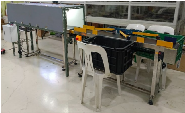
Fig. 9. Developed prototype setup featuring mainly the imaging and sorting conveyors equipped with GP-FL grading constructed custom sorting arms.
