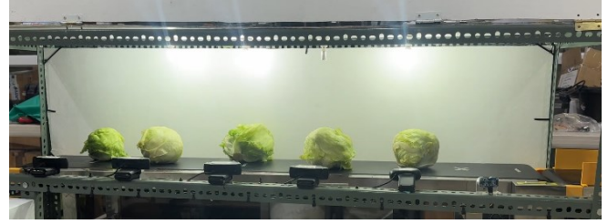
Fig. 8. Camera setup in front of imaging conveyor showcasing placement of iceberg lettuces upon first detection of ultrasonic sensor before sorting.
